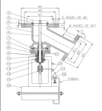
Size Available: - 1" to 6" (DN25 to DN150) Pressure Rating: - class150 Full Bore Flange Standard:-ASME B16.5
